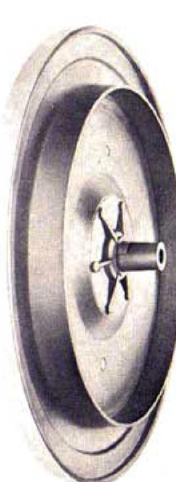
A full 12" diameter provides maximum record support. The die-cast, non-ferrous platter weighs approx. 7 pounds and is machined and precision-balanced to run true and provide optimum performance. Platter mat is deep-ribbed rubber for maximum record protection.
