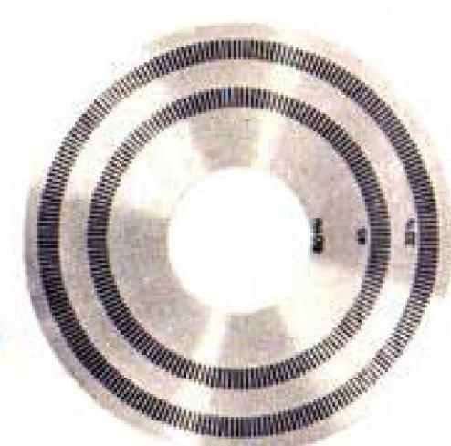
A platter-mounted strobe disc enables precise adjustment of turntable speed when the pitch control is utilized. Markings are provided for both 33 1/3 and 45 RPM speeds.
