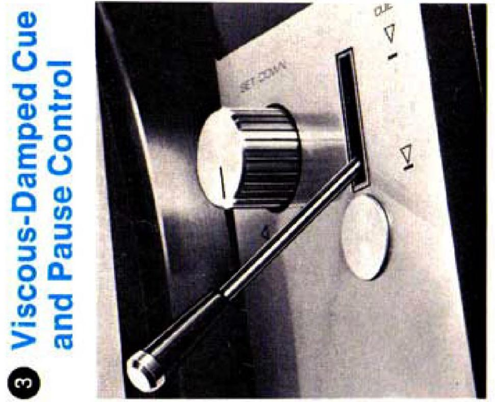
Provides gentle silicone oil-damped tone arm descent. In all other automatic turntables, the anti-skate system tends to move the tone arm outwards while it descends. BSR designed an exclusive positive friction Cue-Clutch that prevents this. After a pause, the 810's tone arm returns to the identical groove, every time. The cueing control can be operated in both automatic and manual modes.
