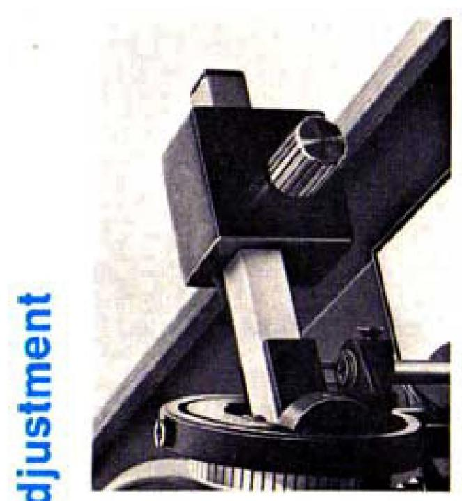
Resiliently mounted gliding one-piece counterweight provides precise "zero-balance" adjustment over a full range of cartridge and stylus masses. A precision micrometer wheel allows continuous infinite stylus pressure settings between 0 and 4.0 grams.
